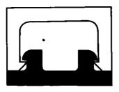
The strength of this joint can be increased by applying adhesive to the mating surfaces before assembly. Even short lengths of an adhesively bonded snap-fit joint cannot be easily slid apart.
