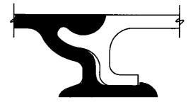
snap-fit joint should only be referenced on drawings. Experienced extrusion designers who are fully conversant with snap-fit production requirements can determine the precise final dimensions.
